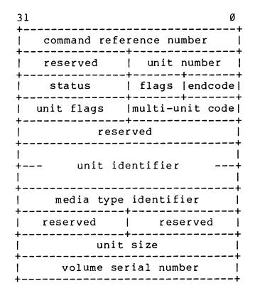
The format and fields of the ONLINE command's end message are identical to the SET UNIT CHARACTERISTICS command's end message; see the field descriptions under that command. The validity of the unit characteristics returned by this command varies with the unit's state. Class drivers can determine which characteristics are valid by examining the values returned in the "status" and "unit identifier" fields.
