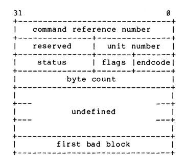
The command reference number and unit number are copied from the command message. The remaining fields are as follows:
